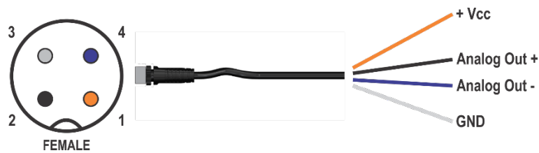
Figure 5 – M12 female output connection
