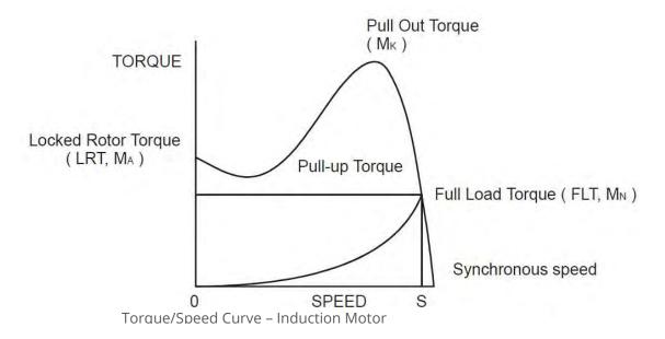
As for each type of motor, so each load coupled to an induction motor has its own speed/torque curve:
