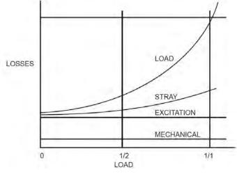
Motor Efficiency/Loss Characteristic
