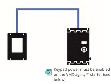
**Enabling Keypad Power:** Scroll to DEVICE menu → KEYPAD menu → KEYPAD PWR = ON
