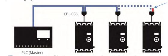
The VMX-agility<sup>™</sup> units must have: a unique Modbus address on each VMX-agility<sup>™</sup> - Use it and identical Parity/Baud rate values on each unit 64 | P
