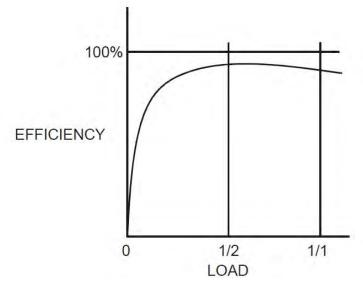
Motor Efficiency/Load Characteristic
