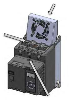
Step 5. Fit flying lead from fan into socket.
