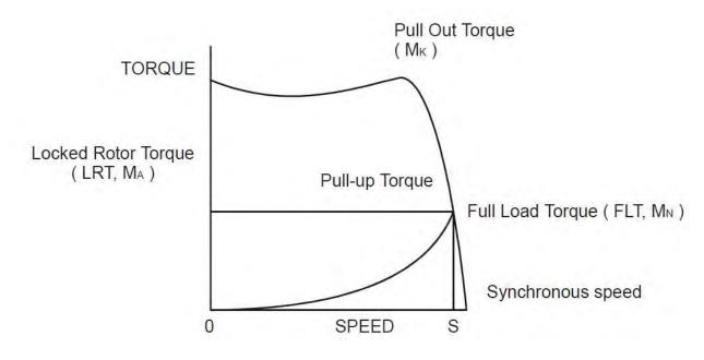
Torque/Speed Curve – High Starting Torque
