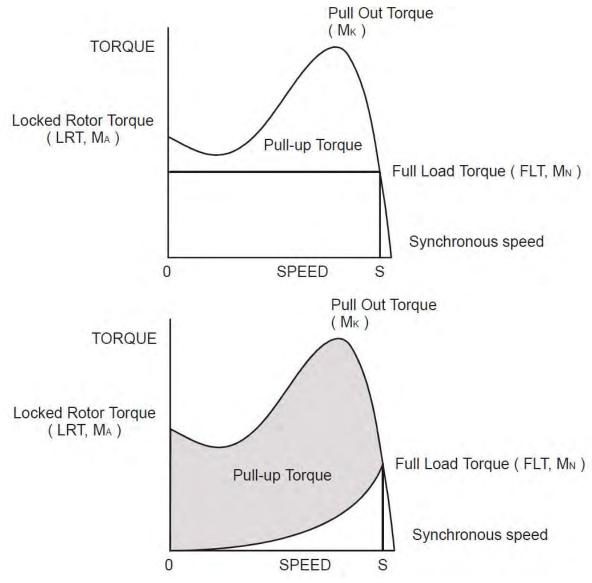
Torque/Speed Curve – Accelerating Torque
