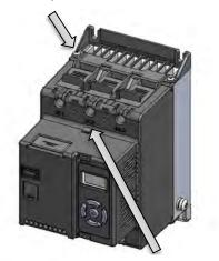
Step 2. Remove blanking plug (x1)
