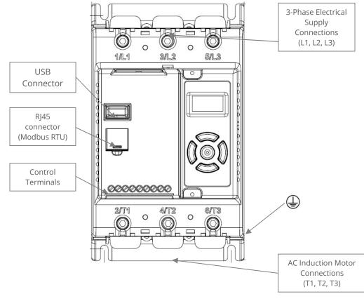
Main Circuit Wiring Diagram
