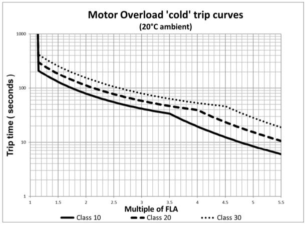
Please note: When the overload has tripped, there is a forced cooling time to allow the overload to recover before the next start.
